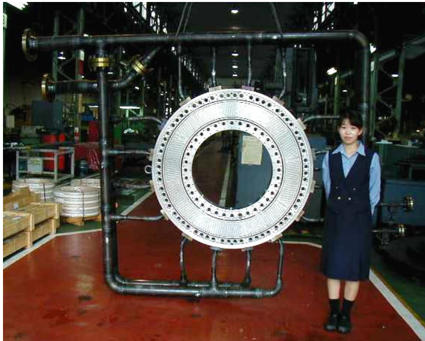
Photo 1 Heat Channel Die of DS1030 (Internally insulated type)
