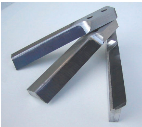
Photo 1 Appearance of JSW-CRA cutter blades
