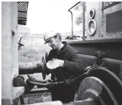
Photo 1. Screw Type Coupler and Uncoupling Operation (Reference: Sited from "Couplers" in Wikipedia)
