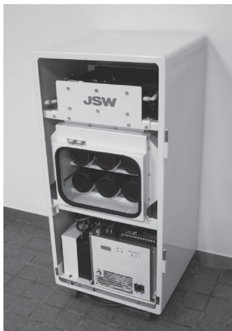
Fig.25 Fuel cell backup power
