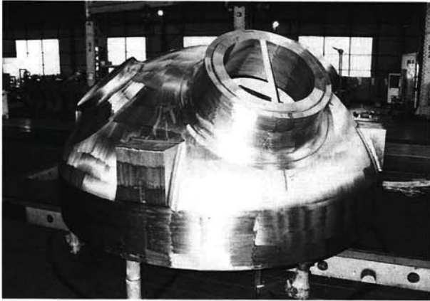
Photo. 10 Integrated forging of primary head for PWR steam generator
