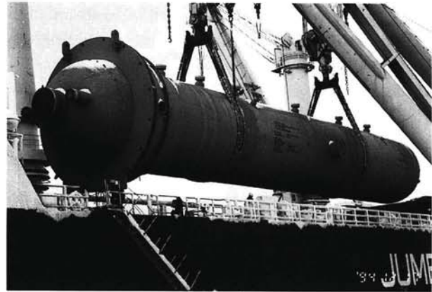
Photo. 13 World large weight reactor for Pernis Refinery of SNR Company (Holland) (material: 12CrMoVTi210, thickness; 273mm, total weight; 1450ton)
