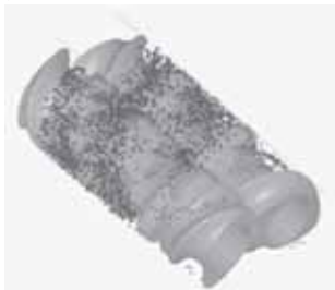
Fig. 4 Marker-particle tracing unsteady analysis in a 3D model.
