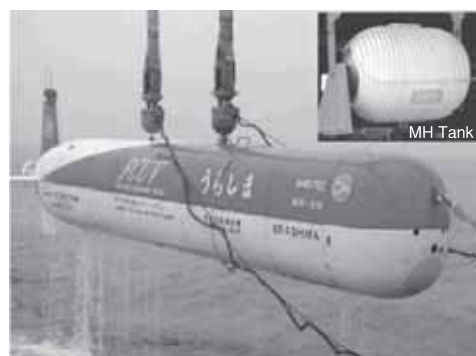
Photo. 11 Fuel cell underwater vehicle "URASHIMA" and MH tank
