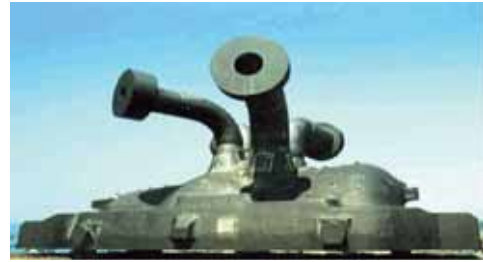
Photo.7 12Cr steel Turbine Casing for USC Plant (Weight : 39.7 ton)
