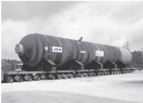
Photo. 8 Land Carriage of 1,200m-tons Reactor by Trailer
