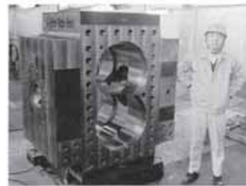
Photo. 8 Casing of large sized gear pump The first GP450T (1986)
