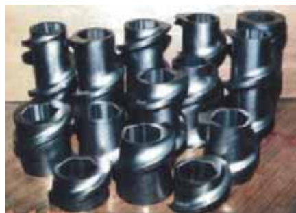
Photo. 12 Screw elements for hexagonal shaft (used until 5 th generation TEX)
