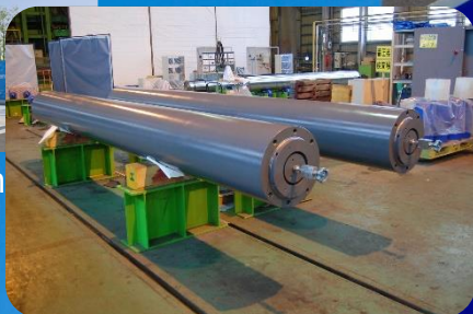
Steel Pressure Vessel for Hydrogen Storage
