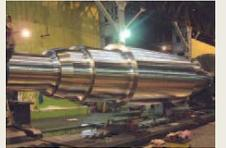
Back-up Roll for Plate Mill
