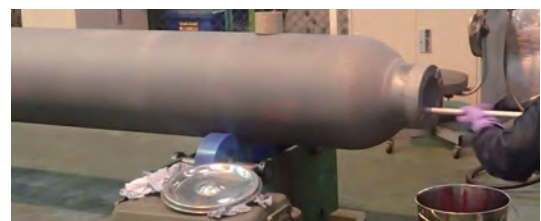
Procedure of Penetrant Test
