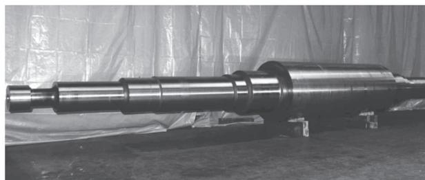
Figure 5 HR1200 trial turbine rotor.
