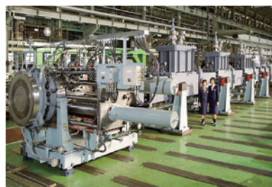
脱揮用大型 TEX Twin Screw Extruder for Devolatilizing Process and Pelletizing Equipment
