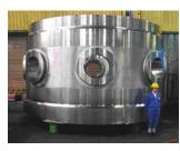
Reactor pressure vessel components
