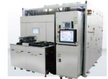
Laser annealing equipment for semiconductors
