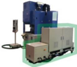
Dedicated molding machine power stabilizer
