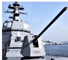
62 Caliber 5-inch Naval Gun (Source: JMSDF)
