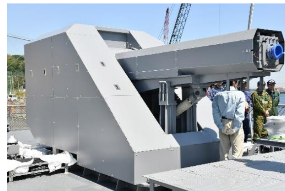
Railgun prototype that was mounted onto test ship Asuka (Source: Self Defense Fleet website)
